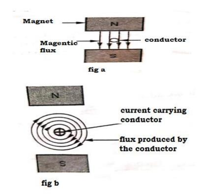
When conductor excited by a separate supply it carries a current in a particular direction. Consider the conductor carries the current away from an observer as shown in the fig.
