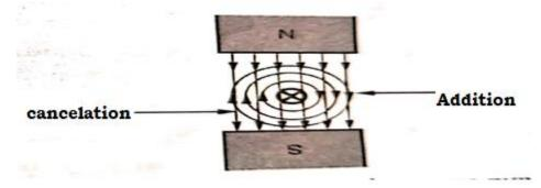
From this, it is clear that on one side (left side) of the conductor, both fluxes are in the same direction, there is gathering of the flux lines as two fluxes help each other.
