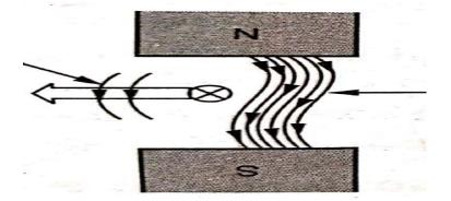
This flux distribution around the conductor acts like a stretched rubber band under tension. This exerts a mechanical force on the conductor which acts from high flux density area towards low flux density area, i.e. From left to right for the case considered as shown in the fig,
