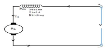
In DC series motor the field winding is connected in series with the source voltage, so the field current **Ise** and the **flux** are not constant.
