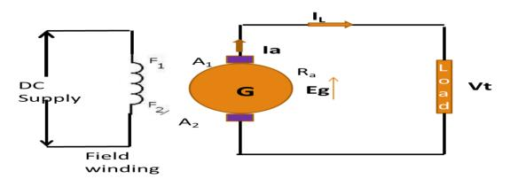
Eg- generated Emf in generator Ia – Armature current R<sub>a</sub> - armature resistance I<sub>L</sub> - Load current Vt- Terminal voltage F1 and F2 – Terminals of field winding
