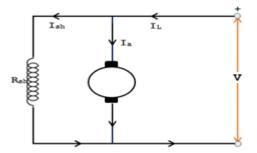
In DC shunt motor the field winding is connected in parallel with the source voltage, so the field current **Ish** and the **flux** are constant in a shunt motor .
