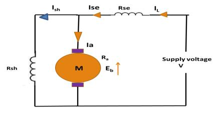
**Long shunt connection Compound Motor** when the shunt winding is so connected that in parallel with the series combination of armature and series field it is called long-shunt
