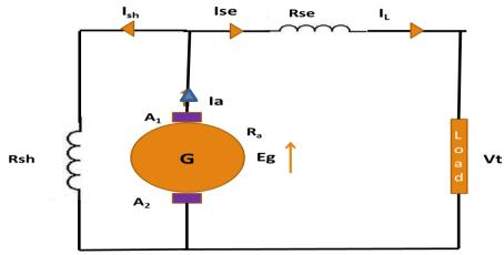
**Long Shunt Compound generator:** The shunt field winding is connected in parallel with the series combination of armature and series field winding.
