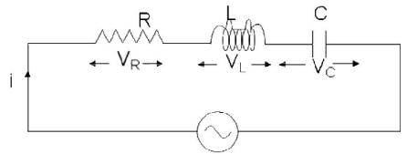
Consider an AC circuit with a resistance R, an inductance L and a capacitance C connected in series as shown in the figure. The alternating voltage v is given by
