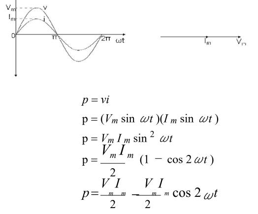
The instantaneous power consists of two terms. The first term is called as the constant power term and the second term is called as the fluctuating power term.
