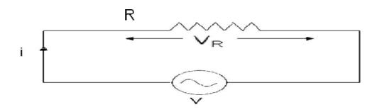
Consider an AC circuit with a pure resistance R as shown in the figure. The alternating voltage v is given by
