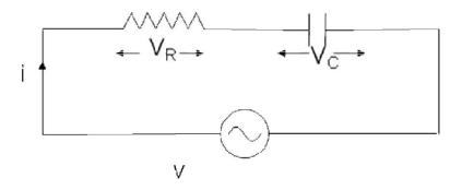
Consider an AC circuit with a resistance R and a capacitance C connected in series as shown in the figure. The alternating voltage v is given by
