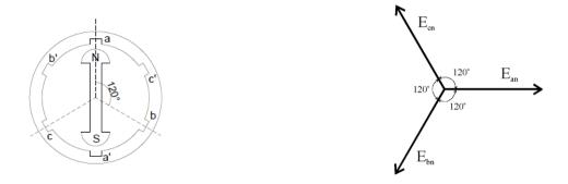
Stator conductors aa', bb' and cc' are mutually displaced by  $120^{0}$ . As the rotor rotates, the stator conductor cuts the flux and hence emf is induced in all 3 conductors.
