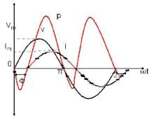
As seen from the power waveform, the instantaneous power is alternately positive and negative. When the power is positive, the power flows from the source to the load and when the power in negative, the power flows from the load to the source. The positive power is not equal to the negative power and hence the average power in the circuit is not equal to zero. From the phasor diagram,
