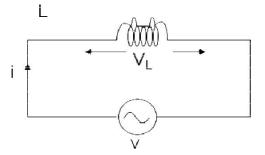
Consider an AC circuit with a pure inductance L as shown in the figure. The alternating voltage v is given by
