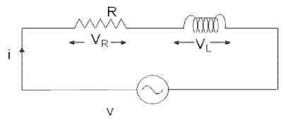
Consider an AC circuit with a resistance R and an inductance L connected in series as shown in the figure. The alternating voltage v is given by
