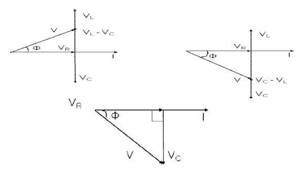
The current I is taken as the reference phasor. The voltage  $V_R$  is in phase with I and the voltage
