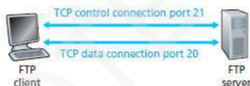
Figure 1.10: Control and data-connections
